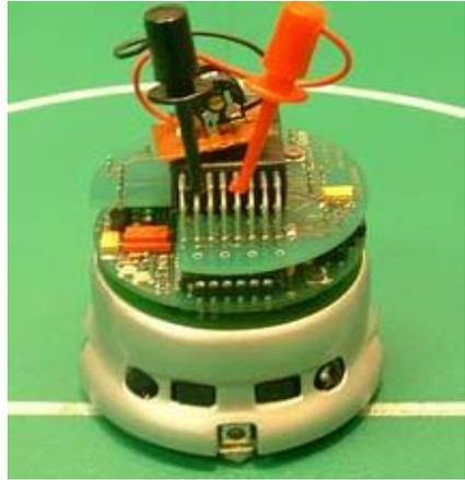
Figure 2 – 14 Connect LED circuit with K213 vision turret
